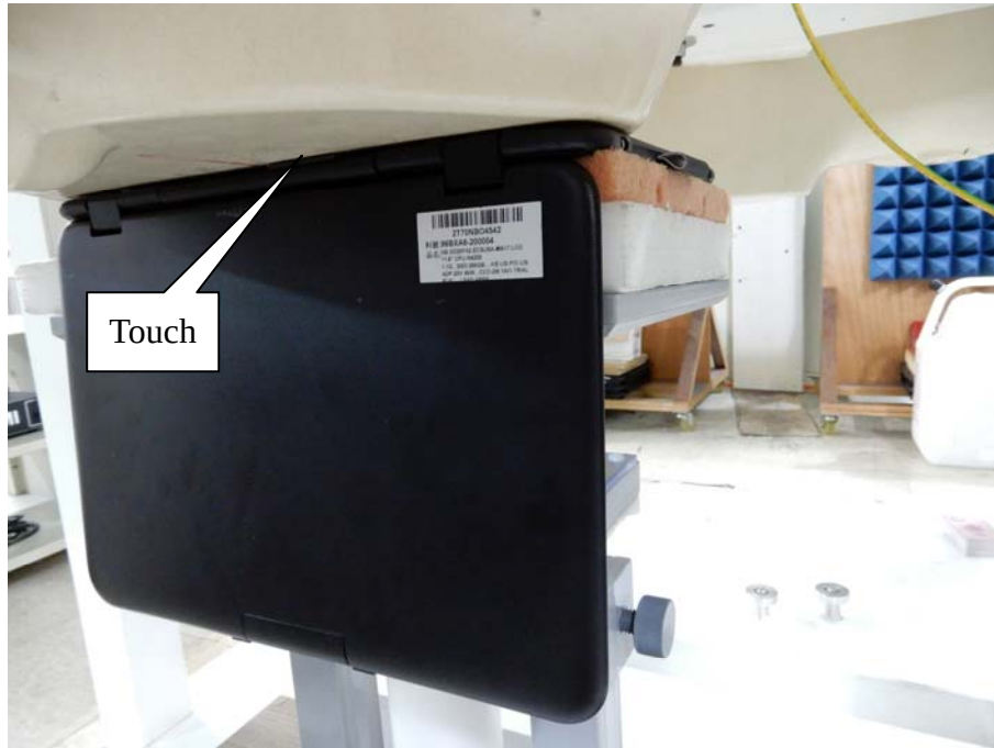
EUT Bottom(NB) – Main Antenna
