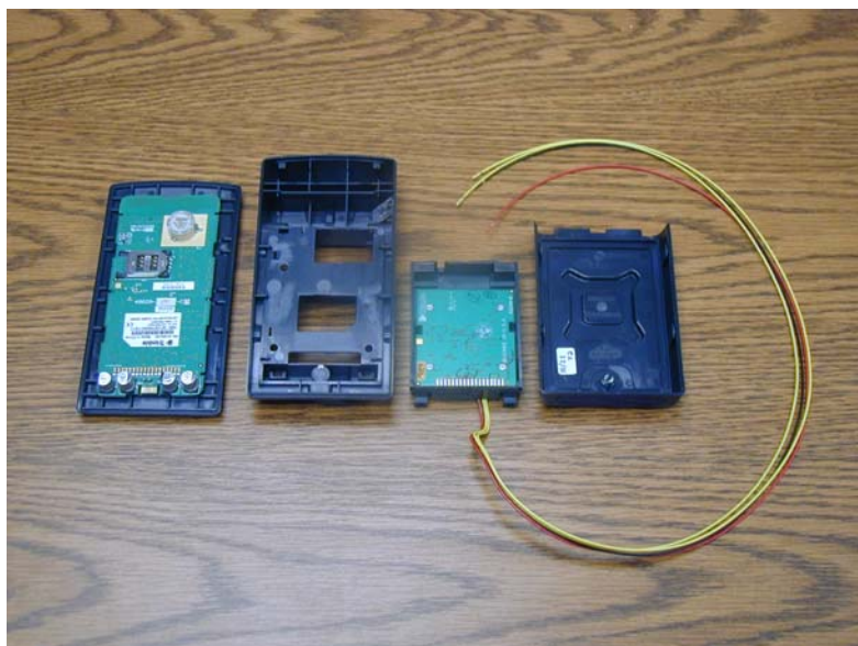
Revised VAM module with revised housing for base and cover.
