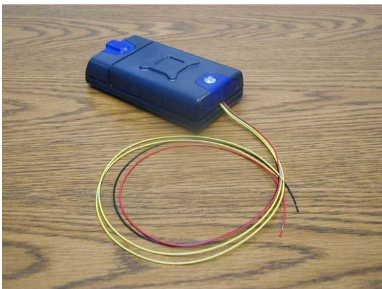
Revised TrimTrac base with VAM module installed and cover in place.
