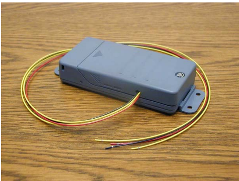
Original TrimTrac base with VAM module installed.
