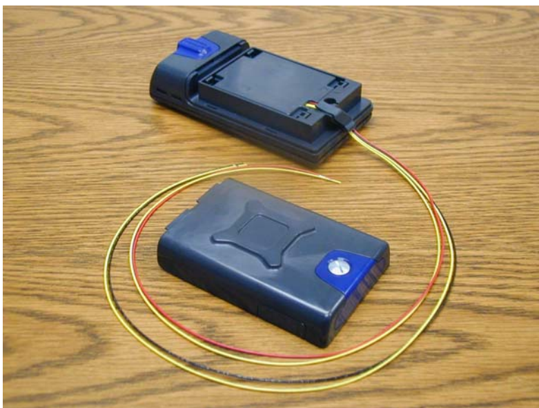
Revised VAM in revised base with cover removed.
