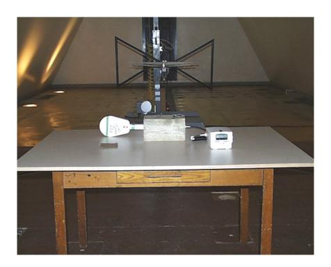
Portable Reader - Radiated EMI Test Setup
