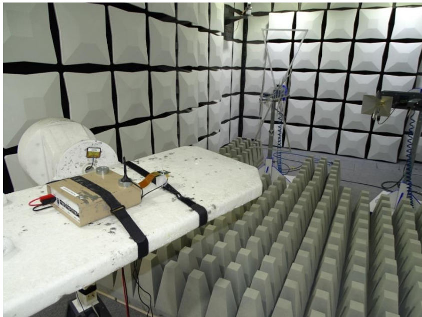
Photo 2: Test setup for radiated measurements above 1 GHz
