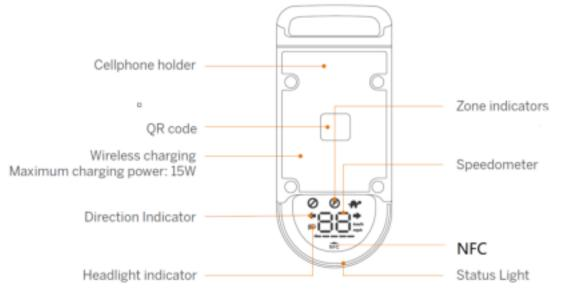
Product Introduction: This product is installed in the dashboard as part of the electric assisted kickscooter, See the above picture.
