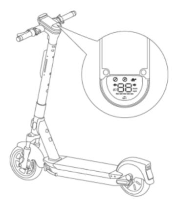
As shown in the figure above, fix the Onboard 15W Wireless Charging on the top of the scooter with screws and connect the corresponding wiring harness.
