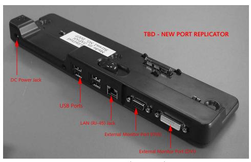
Figure 4-7. Port Replicator rear panel
