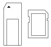
Figure 4-3. Memory Stick (left) and Secure Digital Card (right)
