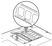
Figure 4-3. Installing a Second Memory Module
