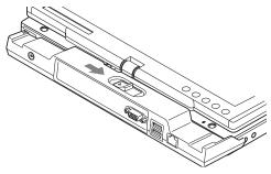
Figure 4-10. Unlatching the Port Replicator
