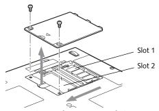
Figure 4-2. Opening the Memory Upgrade Compartment
