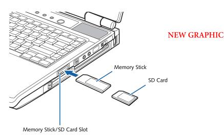
Figure 4-2. Installing a Memory Stick/SD Card
