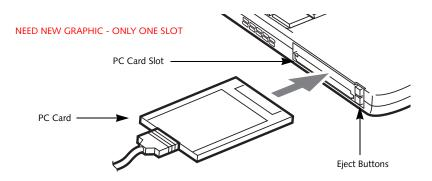
Figure 4-6. Installing/Removing PC Cards
