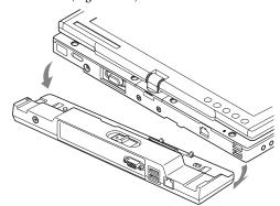
Figure 4-11. Removing the Port Replicator
