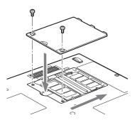
Figure 4-4. Replacing the Memory Compartment Cover
