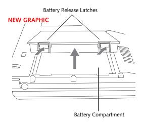
Figure 4-1. Removing the Battery
