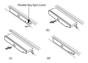
Figure 2-3 Removing/Installing a device in the Flexible Bay
