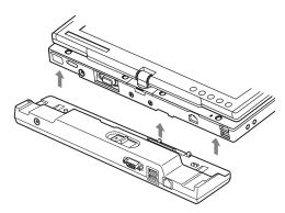
Figure 4-9. Attaching the Port Replicator
