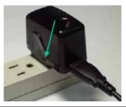
When the LED indicator turns to solid orange, headphone is charging. When the LED indicator goes off, the headphone is fully charged. The headphone may take 2.5 hours to fully charge.
