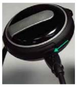
Connect the other side of this USB cable to PC or the AC adaptor.
