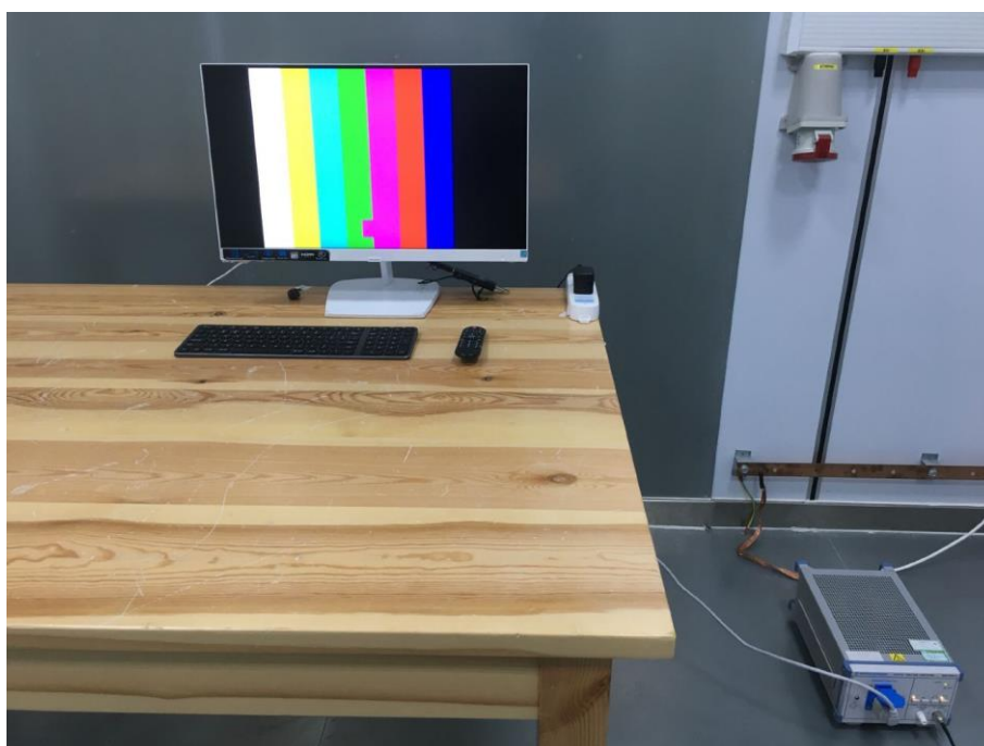
Fig. 4 Power line conducted emission setup photo
