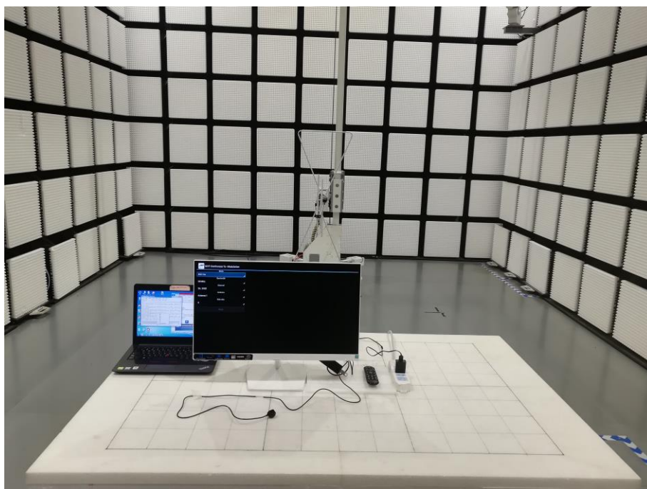
Fig. 2 Radiated emission setup photo(30MHz-1GHz)
