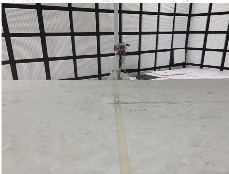
Radiated spurious emission Test Setup-2 left ear(Above 1GHz)
