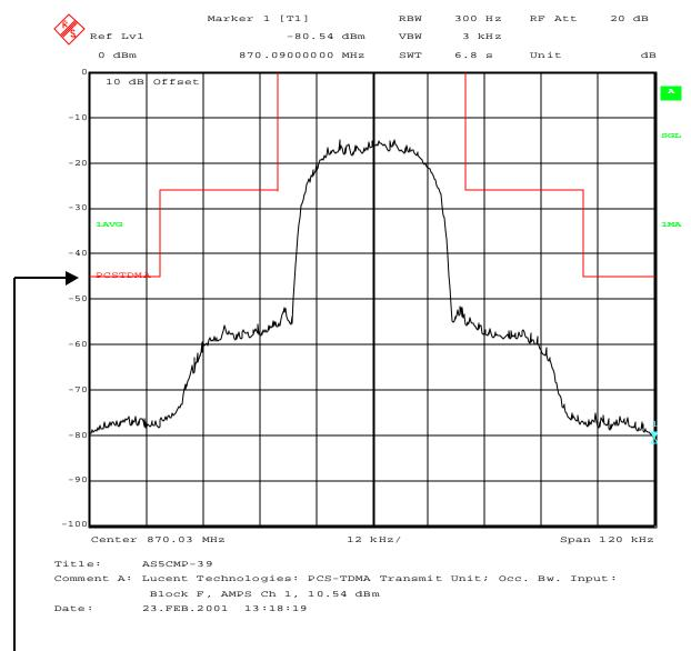
Occupied Bandwidth; Antenna Terminal; Block F; PCS Ch 1498
