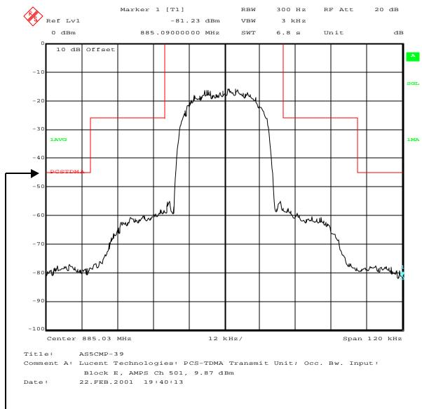
Occupied Bandwidth; Antenna Terminal; Block E; PCS Ch 1331
