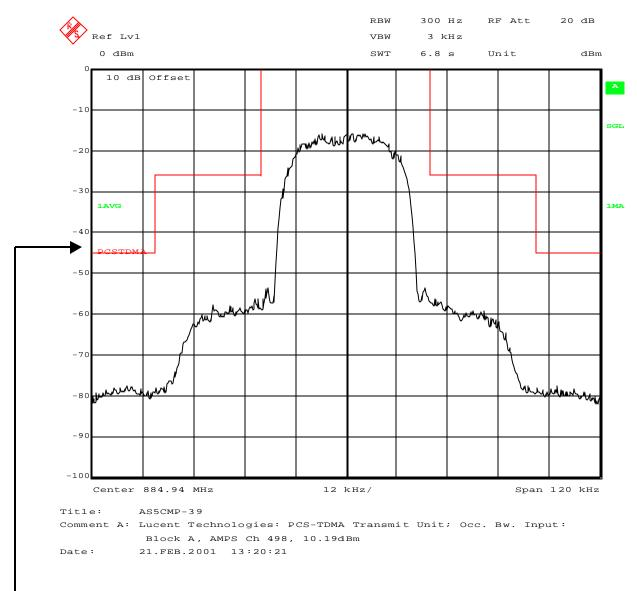
Occupied Bandwidth; Antenna Terminal; Block D; PCS Ch 583
