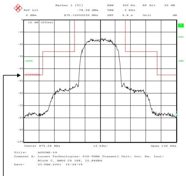
Occupied Bandwidth; Antenna Terminal; Block C; PCS Ch 1998
