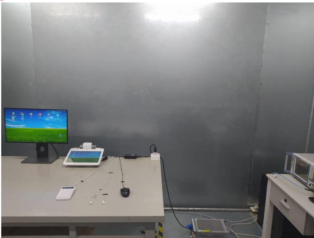
Fig. 3 Power line conducted emission setup photo
