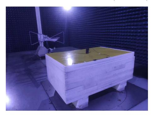
**Photo of Radiated Emission Measurement (Above 1GHz)**
