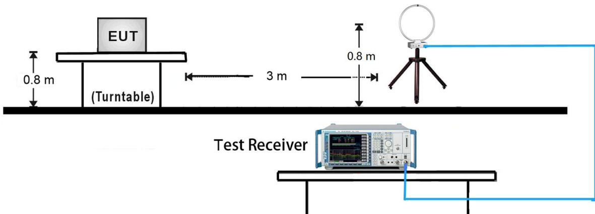
30MHz ~ 1GHz Test Setup:
