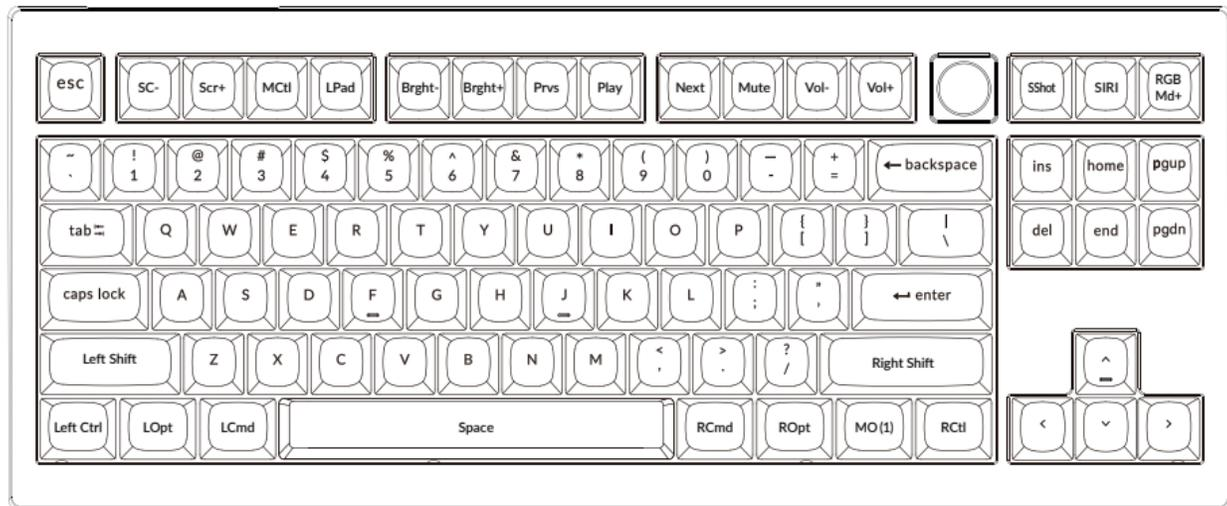
**LAYER 1:** This layer will be activated when your keyboard's system toggle is switched to Mac and press the fn/MO(1) key.
