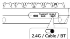
Press fn + 1 (for 4 seconds) and pair with device named Keychron V3 Max.
