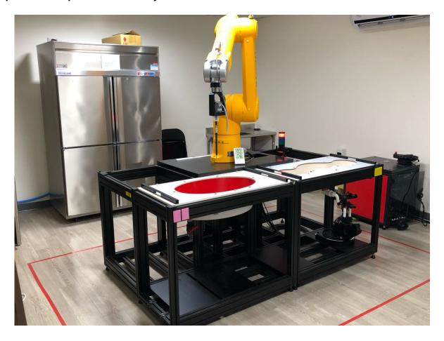
Liquid depth in the flat Phantom (≥15cm depth) HSL(5GHz)
