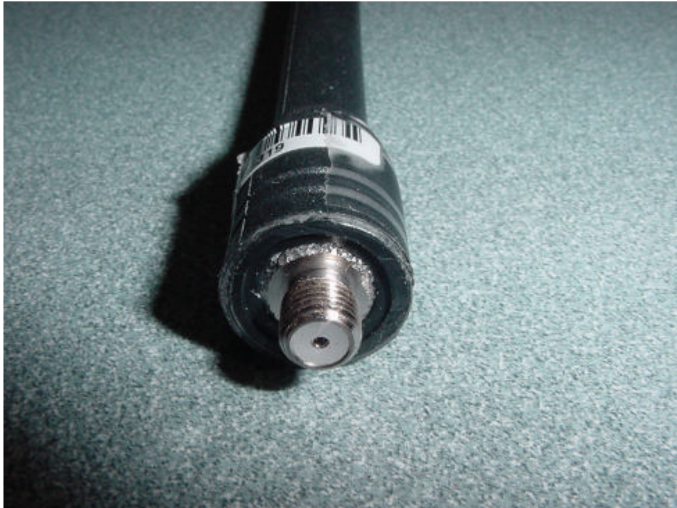
PHOTOGRAPH 34: ANTENNA CONNECTOR (MURS-25)
