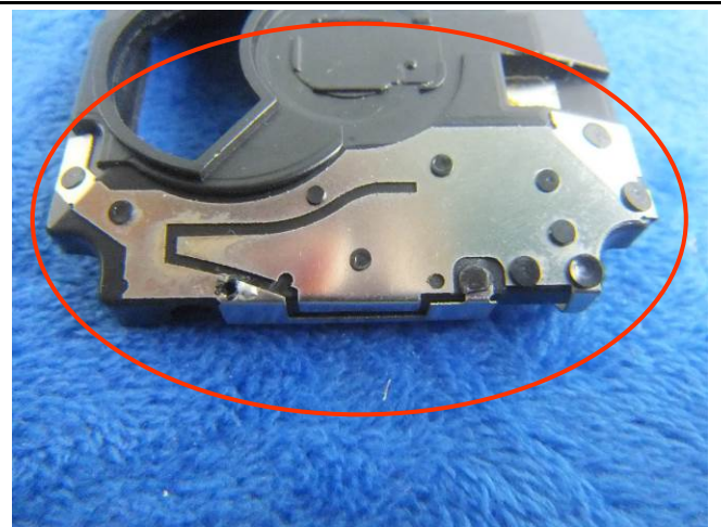
GSM/PCS Antenna View
