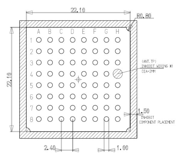
order to easily rework the GE865 is suggested to consider on the application a 1.5mm Inhibit area around the module.
