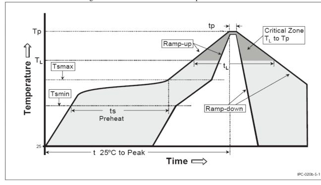
The following is the recommended solder reflow profile
