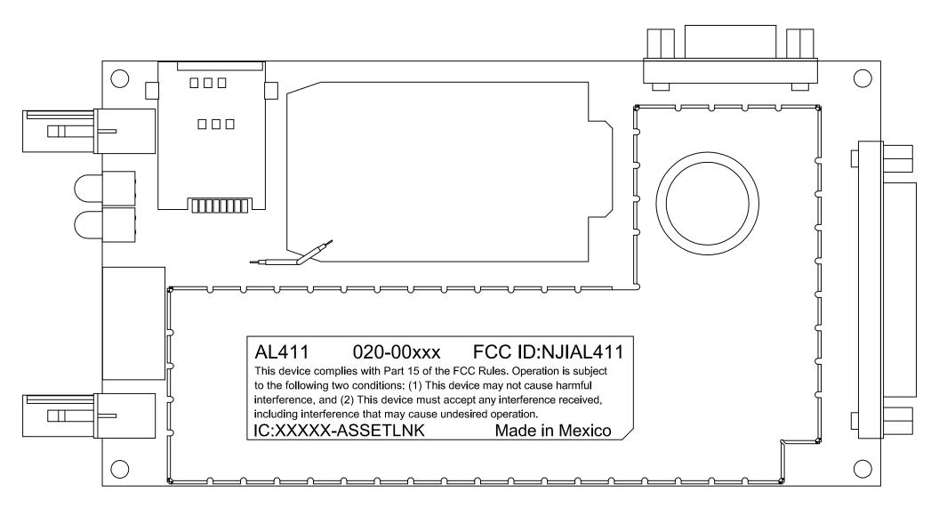
On the Model Number: typeface shall be 10 point Arial Bold, lettering shall be black on a white or silver background. On the FCC ID are: typeface shall be at least 10 point Arial Bold, lettering shall be black on a white or silver background. On the warning area: typeface shall be 6 point Arial Normal on a white or silver background.
