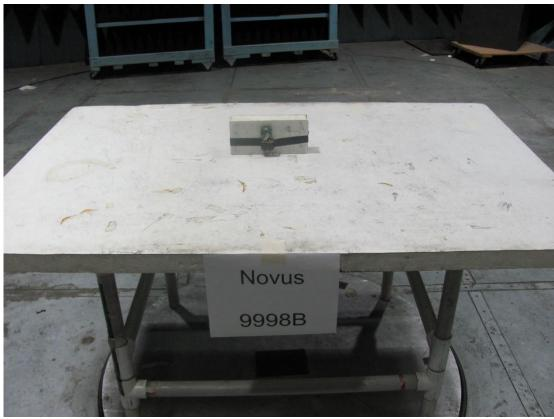
The EUT was taped to a foam block in order to change the axis of rotation.
