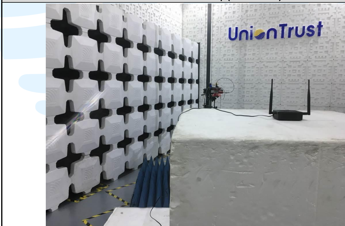
Radiated emission Test Setup (Above 1 GHz)
