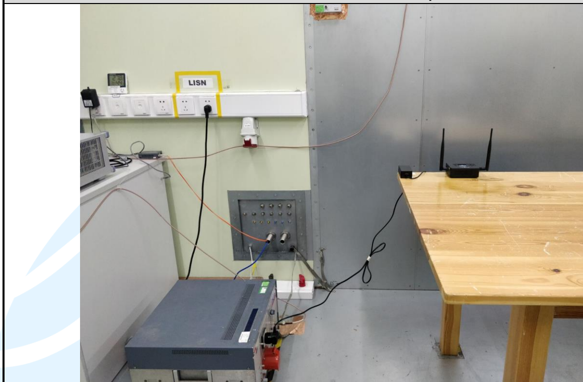
Conducted Emission Test Setup
