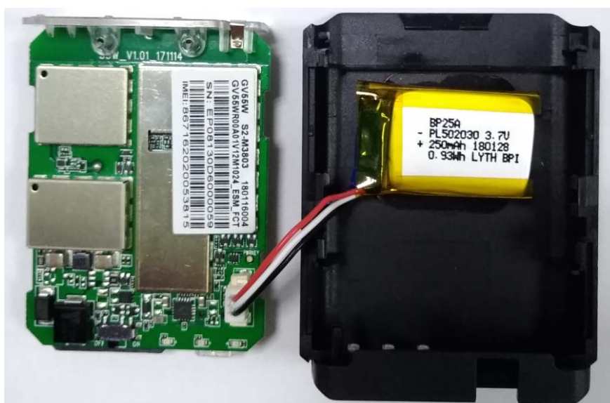
Figure 6. Backup Battery Installation
