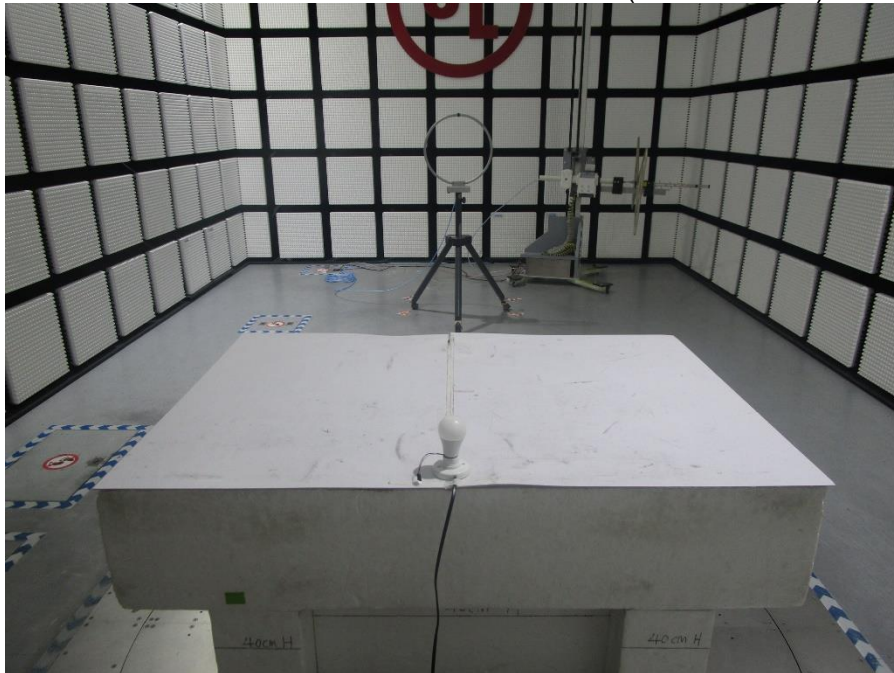
RADIATED RF MEASUREMENT SETUP (Below 30MHz)
