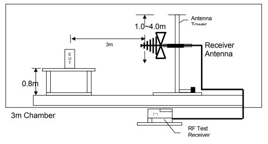
Test setup of radiated emissions upto 1GHz
