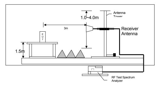
Test setup of radiated emissions above 1GHz
