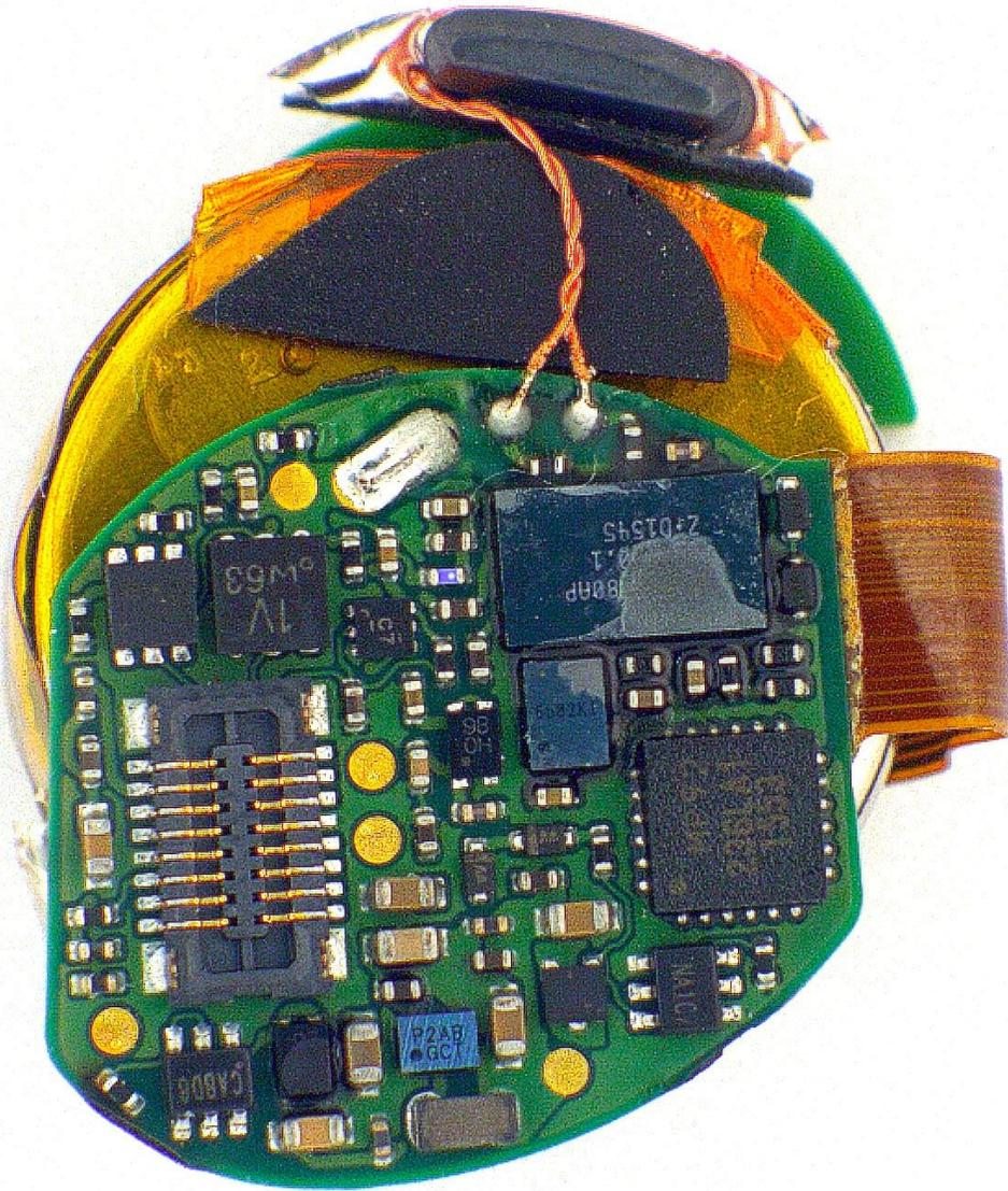
PC board top view (NFMI antenna on top)
