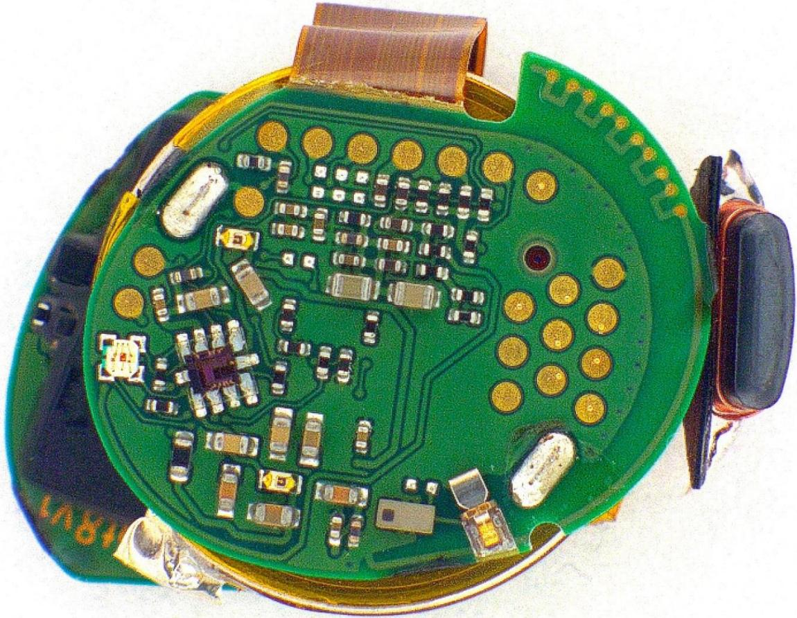
PC board bottom view (NFMI antenna on right, Bluetooth LDS antenna pickup point at 5 o'clock position)
