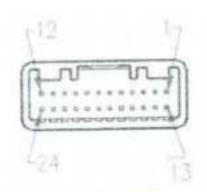
Pin definition of tire pressure monitoring control module assembly in the above figure
