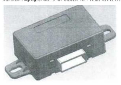
The appearance of the connector on the TPMS receiver is shown in the figure. The connector model is TE: 1318853-2, and the detailed pin definition is shown in the table. The corresponding connector model is TE: 1318917-1
