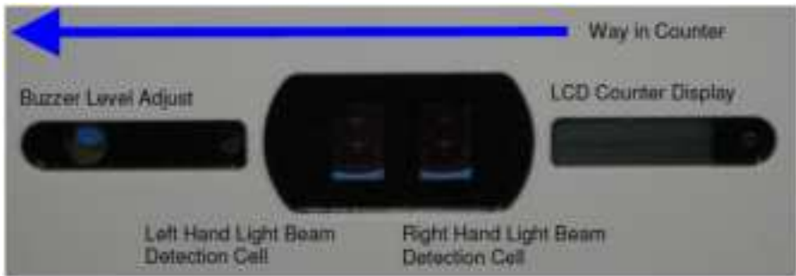
Figure 4.6: People Counter View when facing light barrier and counter display
