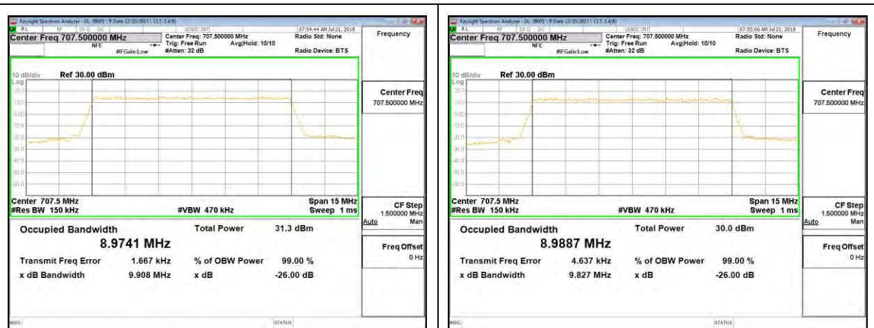
LTE B12 10MHz QPSK Mid Channel RB50-0
