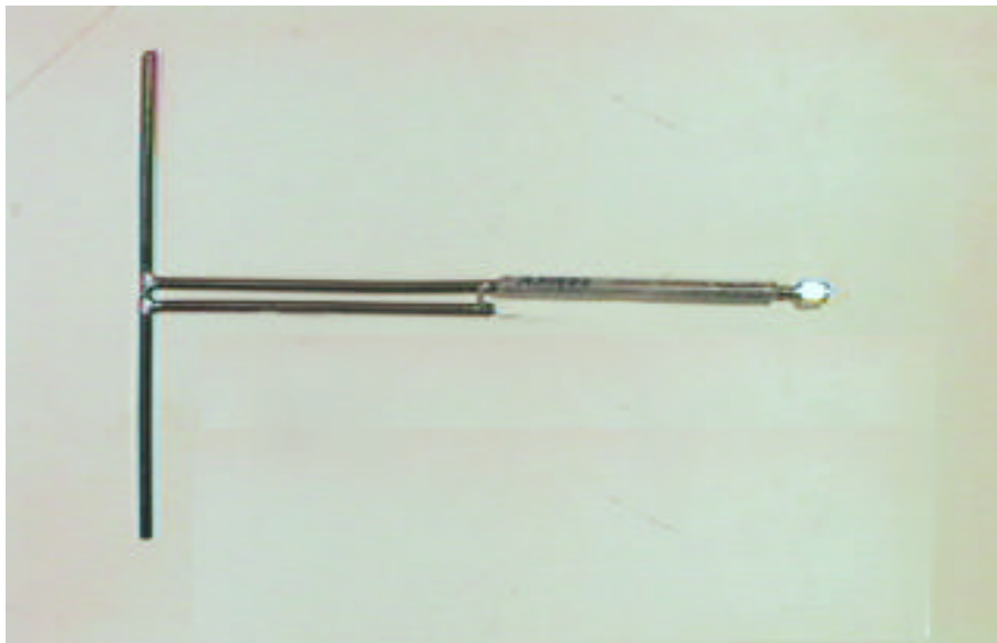
Reference Dipole Antenna Used for ERP Measurement
