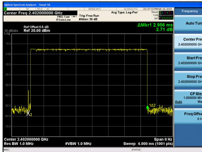
2DH5 on time (Count Pulses) Plot on Channel 00
