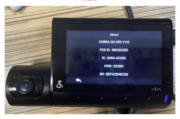
Note: E-label include FCC ID, IC ID, HVIN, SN and the other information that is not on the device label.
