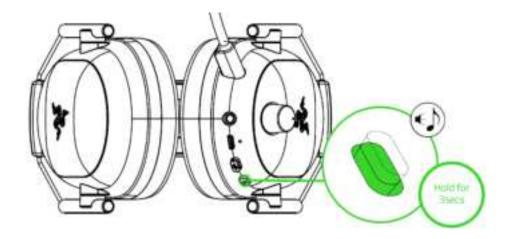
3. Wait until the status indicator briefly becomes static blue indicating that the headset is now connected to the USB wireless transceiver.
