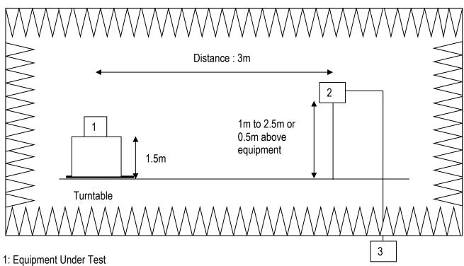
2: Measurement antenna with tilt for variation from 1 to 2.5m or 0.5m above top of equipment
