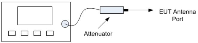
The measure is realized in conducted mode and average output power spectral density is measured with a spectrum analyzer:
