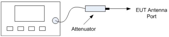
The measure is realized in conducted mode and average output power is measured with a spectrum analyzer:
