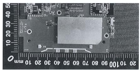
2. The Thread module has two antennas, but the PCB antenna is not connected with other components, so there is no signal transmission of the PCB antenna. We just reserved the position in advance.
