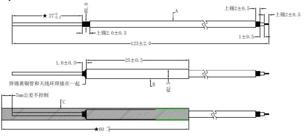
Figure 1 Physical dimension (mm)
