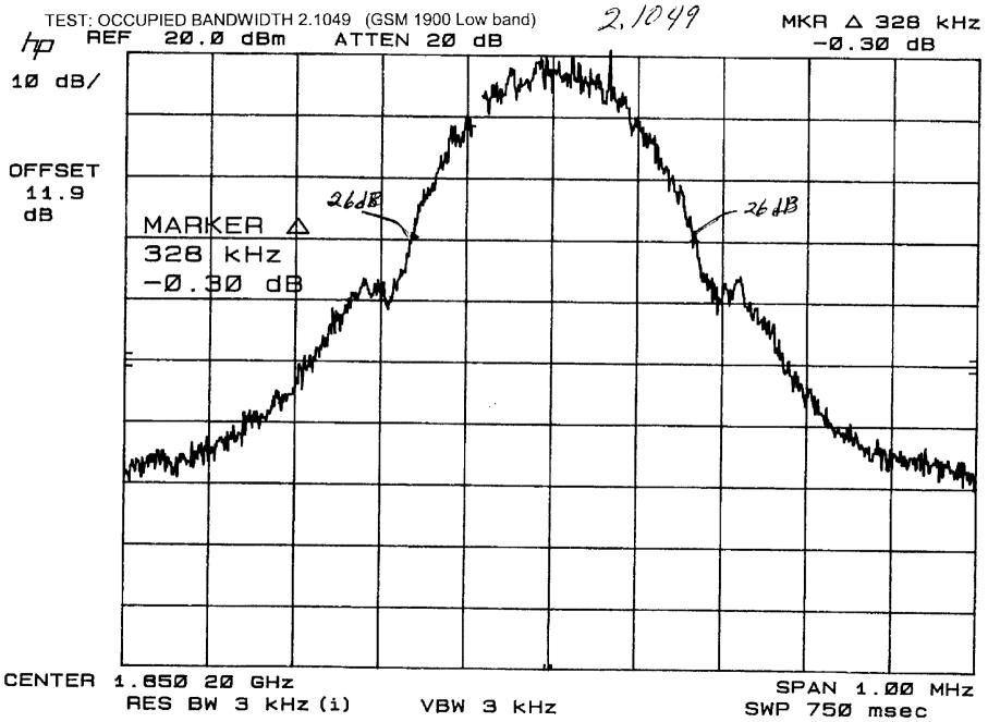
**CUSTOMER: SIEMENS** EUT: "S46" FCC ID:PWX S46 TEST: OCCUPIED BANDWIDTH FCC Part 2, Para. 2.1049 (GSM1900 Mid Band)
