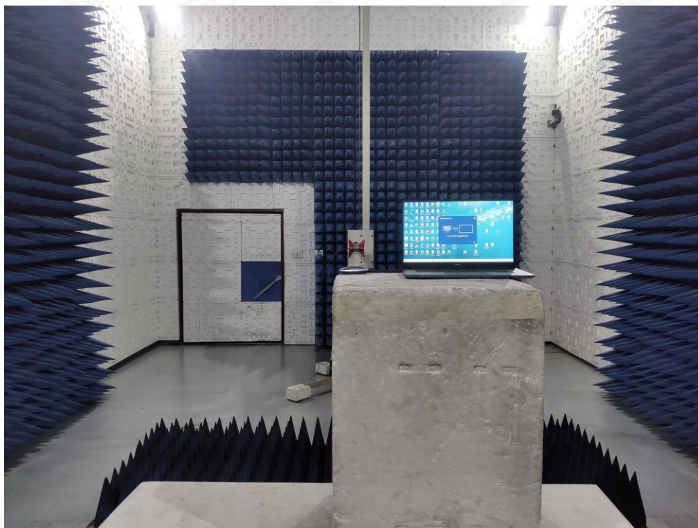
FCC RADIATED EMISSION TEST SETUP ABOVE 1GHZ
