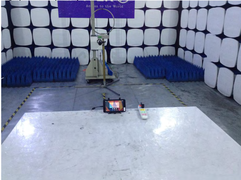
Photograph 2: Set-up for Spurious Emissions for 30 - 1000MHz
