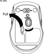
2 Insert the included AAA batteries into the battery compartment. Make sure that the + and - signs match the symbols in the compartment.
