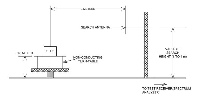
The spectrum was searched up to the 10th harmonic of the fundamental frequency of operation.
