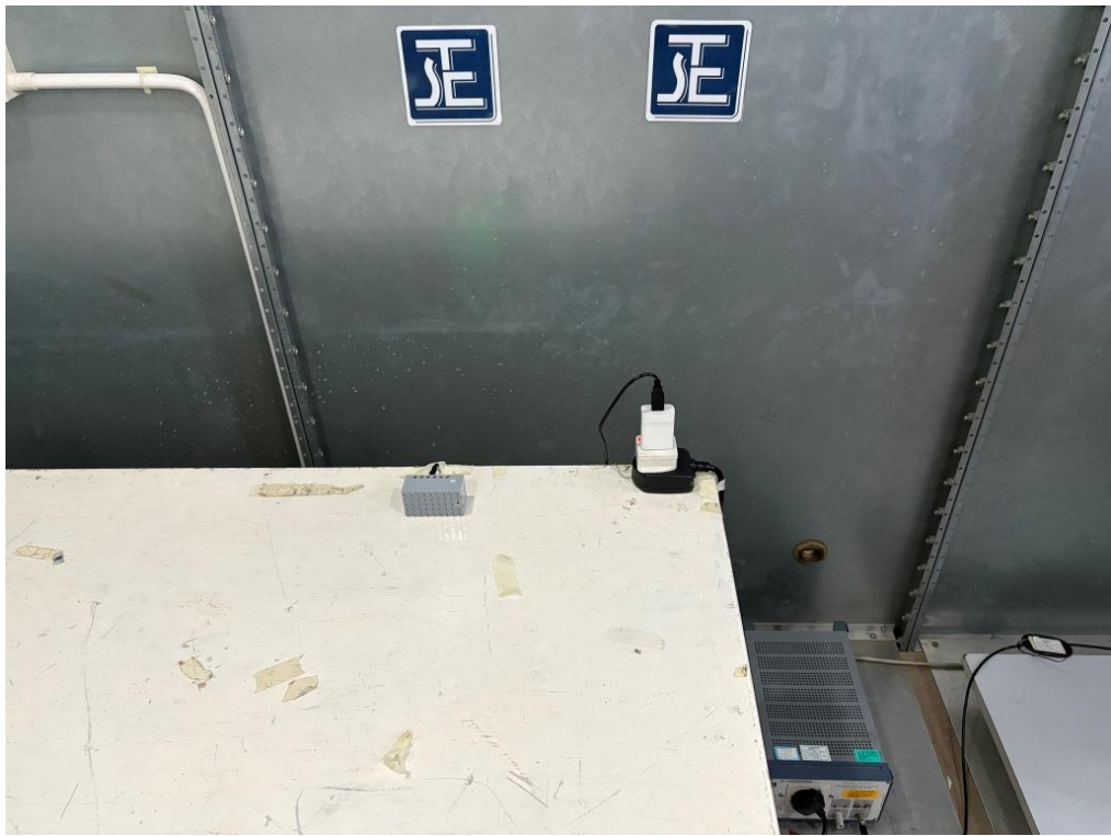
Measurement of Conducted Emission Test Set Up
