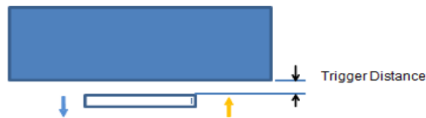
Picture: Proximity sensor triggering distances assessment (Back side)->
