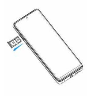
To eject SIM or MicroSD cards, insert your SIM eject pin into the small hole next to the card tray.
