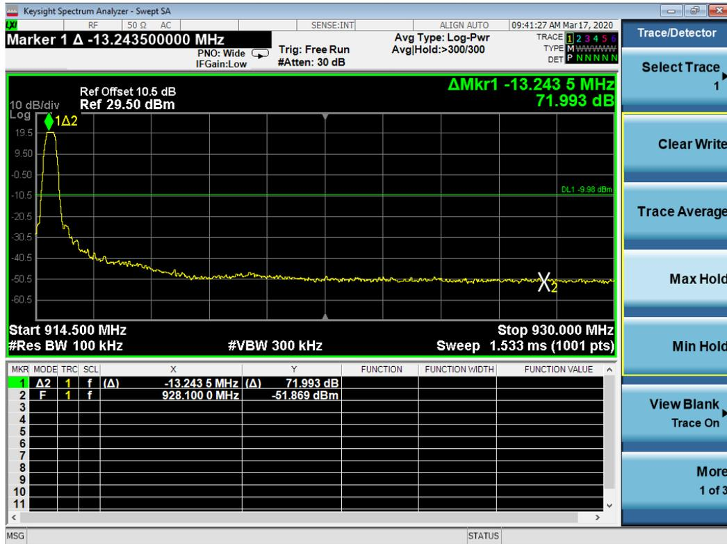
Screen Capture from the spectrum analyzer: Lower Band Edge (125 KHz Hopping)
