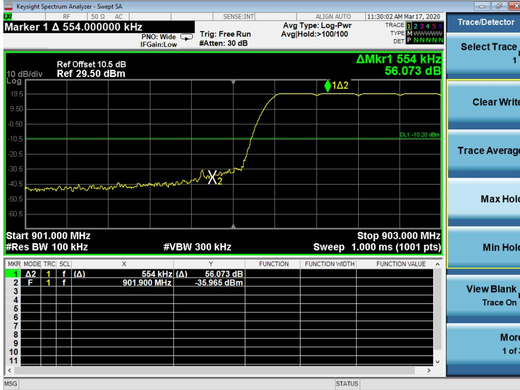
Screen Capture from the spectrum analyzer: Upper Band Edge (125 KHz Hopping)
