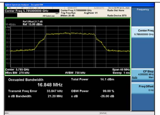
802.11a UNII 3 BAND 26dB Bandwidth (CH 157)
