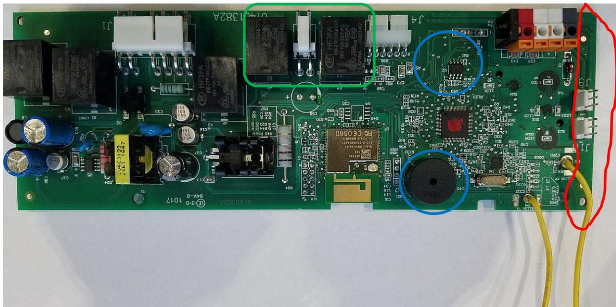
Circled in red is the area of the board added with the new PCB connectors.
