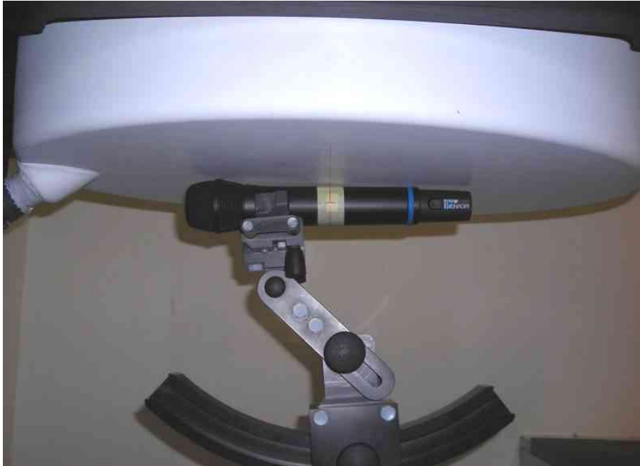
Figure 9 – Tested device position: with the Right side against the phantom
