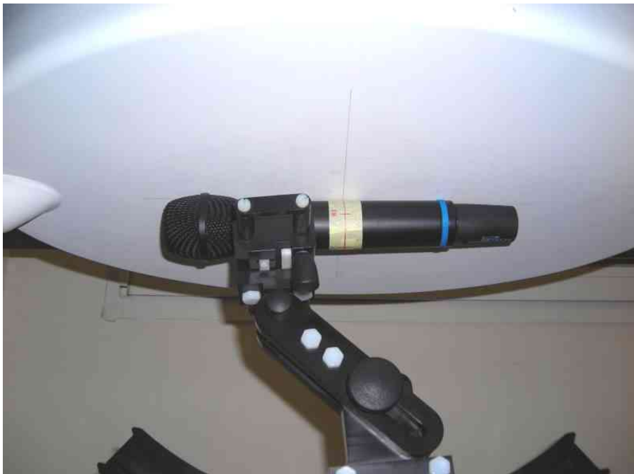
Figure 8 – Tested device position: with the Rear side against the phantom
