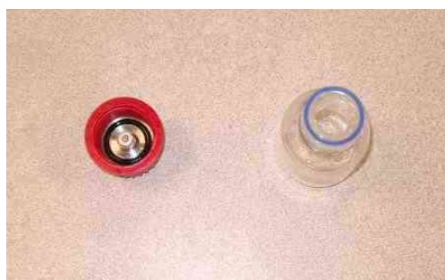
Figure 18 - Open coaxial probe with the bottle cap
