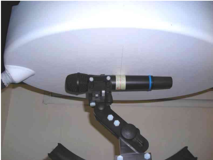
Figure 7 – Tested device position: with the Front side against the phantom
