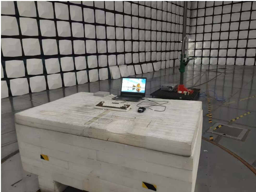
Radiated Emission 9k-30MHz Perpendicular View
