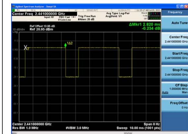
Modulation: GFSK DH5 2441
