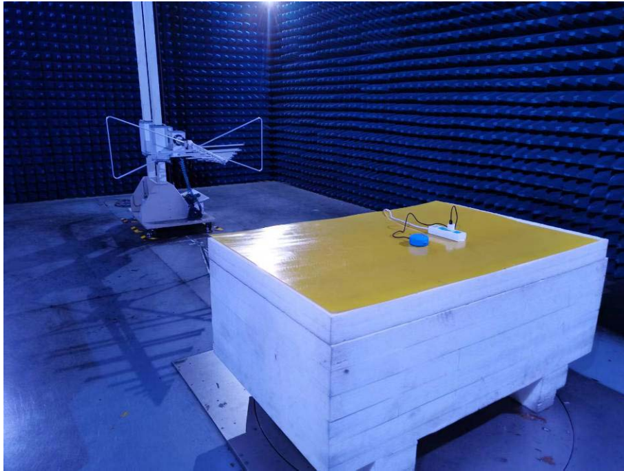
Photo of Radiated Emission Measurement Below 1GHz
